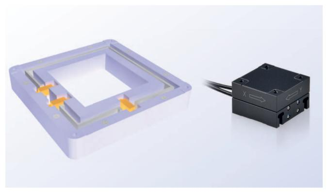
In a parallel-kinematic structure, all drives act on the same moving platform so that the individual axes have the same dynamic behavior. Consequently, higher dynamics and higher scanning frequencies, improved guiding accuracy, repeatability and stability can be achieved than with serial axes systems
