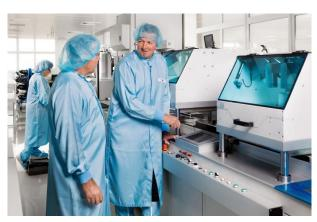
Abb. 3 Workplace for manufacturing PICMA® multilayer actuators in an ISO class 6 cleanroom at PI Ceramic
