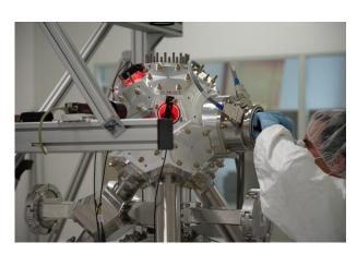
Abb. 4 Multi-axis positioning system for X-ray spectroscopy, manufactured in an ISO class 7 cleanroom at PI miCos in Eschbach, Germany
