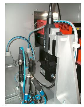
Fig. 8 Integration of the laser vibrometer in the a bench (Image: Pari Pharma/Polytec)
