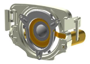
Fig. 4 The annular piezo is directly glued to the metal ring of the diaphragm. When the a.c. voltage is applied, the piezo element oscillates with a frequency of 120 kHz (Image: Pari Pharma/PI)
