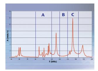
Fig. 7 Quality control with the laser vibrometer: example of the frequency spectrum of a diaphragm (Image: Pari Pharma)
